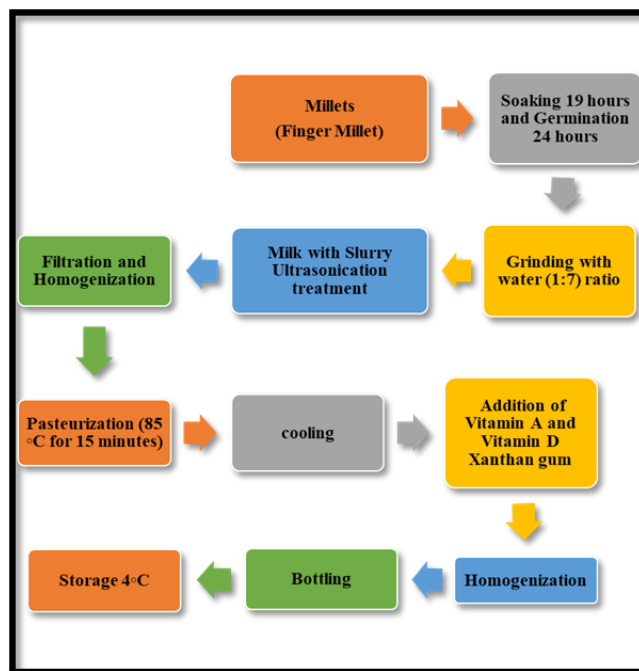
Fig. 1: Process flow chart for the preparation of unfortified and vitamin fortificants finger millet milk
